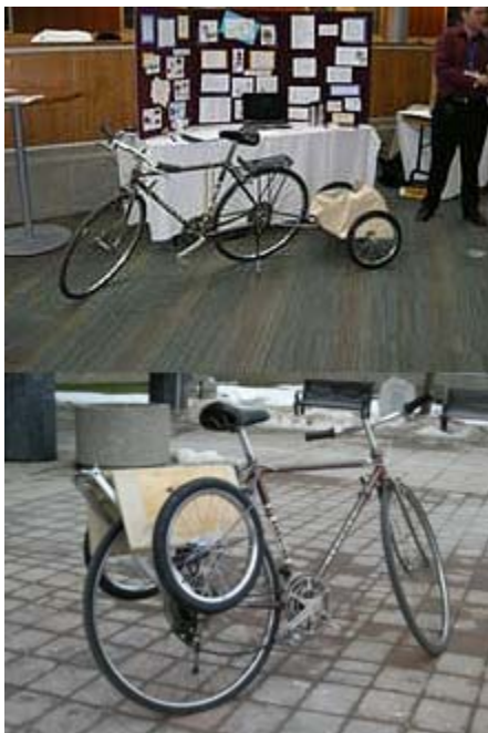
Kettel and Minkhorst's trailer, shown both unfolded (top) and folded. (McMaster Engineering)
